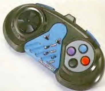
The new Logipad joystick has six fire buttons and an eight-way thumb control.
